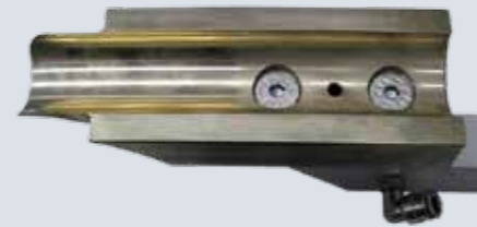
Wiper die with lubricating hole
