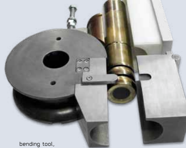
bending tool, mandrel and wiper die
